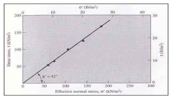
Fig3. Direct shear test
